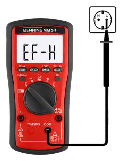
Figure 15: External conductor or phase testing
