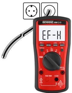
Figure 14: Non-contact phase testing
