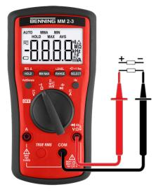
Figure 11: Resistance measurement or continuity test
