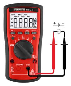
Figure 9: Voltage or frequency measurement
