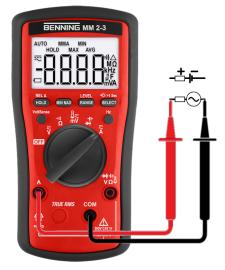
Figure 10: Current or frequency measurement
