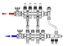
Correct installation of manifold with flowmeter
