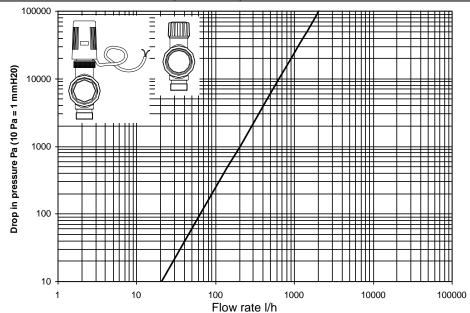
Analytical procedure to determine the drop in pressure for liquids with  $\rho \cong 1 \ kg/dm^3$
