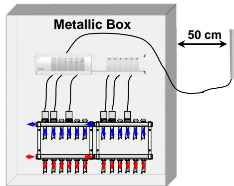
\* For maximum radio sensibility, the active antenna must be placed at a minimum of 0.50 cm of any metallic surfaces (Electrical Box) or vertical metallic pipes.
