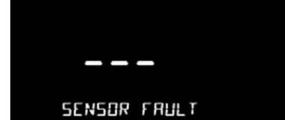
In case of the error indication, please check the proper functioning of the connected probe.
