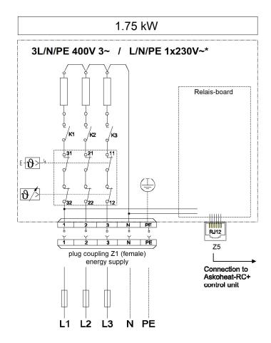
\* for single-phasing (1x230V~), L1, L2 and L3 use external jumper
