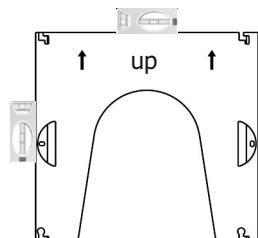
2. Label the selected drill holes at the specified markings with a pencil.
