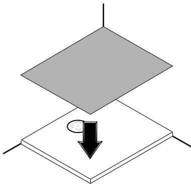
**VARNING:** SKYDDA ALLTID BRICKANS YTOR MED KARTONG ELLER POLYSTYREN VID INSTALLATION AV SJÄLVVA
