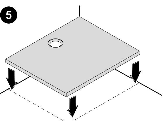
PLACERA PLATTAN OCH KONTROLLERA ATT AVLOPPET ÄR I RÄTT LÄGE
