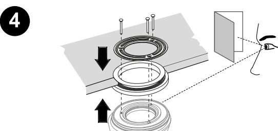
MONTERA PACKNINGEN OCH SKRUVA I METALLRINGEN
