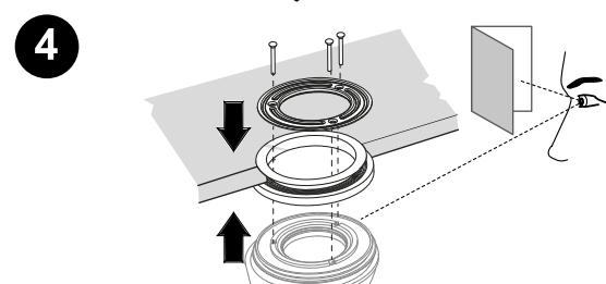
NAINSTALUJTE TĚSNĚNÍ A NAŠROUBUJTE KOVOVÝ KRUŽEK
